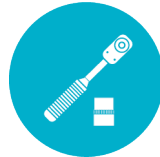
Torque wrench 10 - 30 Nm with socket for WS 13
