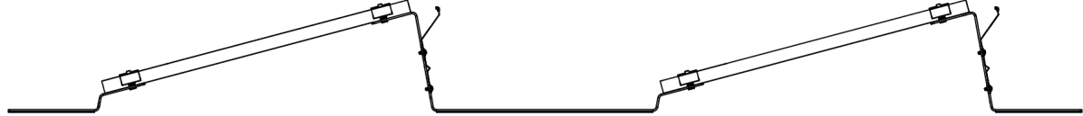
SYSTEM S15 | 790 MM ROW SPACING | 18° SHADING ANGLE
