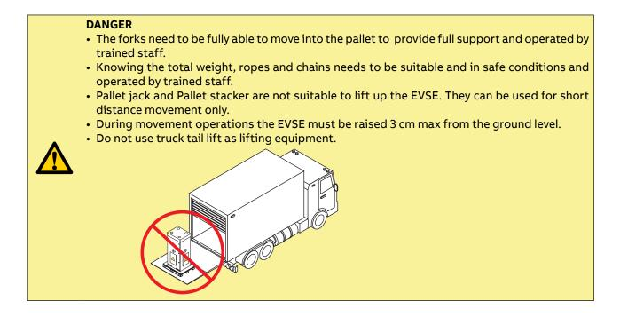
• Check that the pallet is not damaged. If there is damage, contact the responsible Health and Safety manager for the site to get instructed on how to unload the EV Charger and move it in a safe way. Pay particular attention to the position of the wheels of the Pallet jack and pallet stacker to avoid damaging the pallet.
