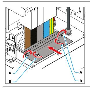
• Close the sliding plate using the 2 side screws (A).
