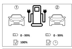
When the EVSE is configured for sequential power allocation, it can serve one EV at a time with DC fast charging.
