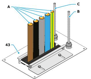
**Risk of pinching or crushing of body parts** Make sure that cables do not get trapped between the EVSE and the base and that are aligned to the AC and PE connection terminals.
