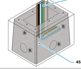
foundation (45) using the 4 entry holes (B) and applying cable slack of each cable 700 mm.
