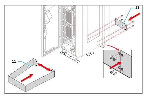
• In order to install the base covers (11), repeat the operations described in the "Remove the border covers" section in reverse order.
