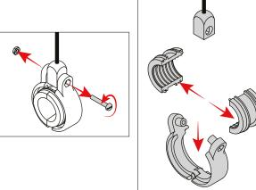
• Install the "Clamp insert" on the charging cable (at 8.2 in (250 cm) starting from the EVSE) and lock it in position by inserting the 2 springs.
