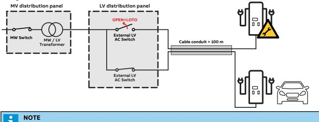
Multiple chargers – AC lines in common cable conduit > 100m length – an AC line charged
