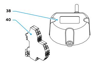
The tilt sensor is generally closed and opens when the tilt exceeds 10° in any direction, for example if a vehicle impacts against the EVSE. It can be used to open (in combination with undervoltage release circuit) the upstream protections keeping the EVSE de-energized.
