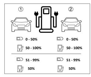
One EV connected => 100% of the power Two EV connected => 50% of the power
